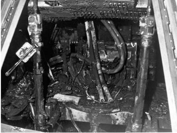
**Fig. 5.23** *Apollo-1* cockpit after the fire of 27th January 1967 (<http://www.space.com/10674-apollo-1-fire-nasa-disaster.html>)
