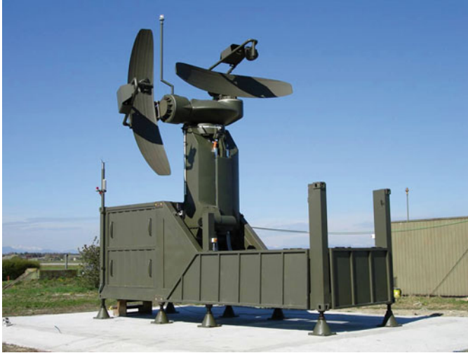
Fig. 1.20 Precision approach radar. (Source: Selex System Integration)
