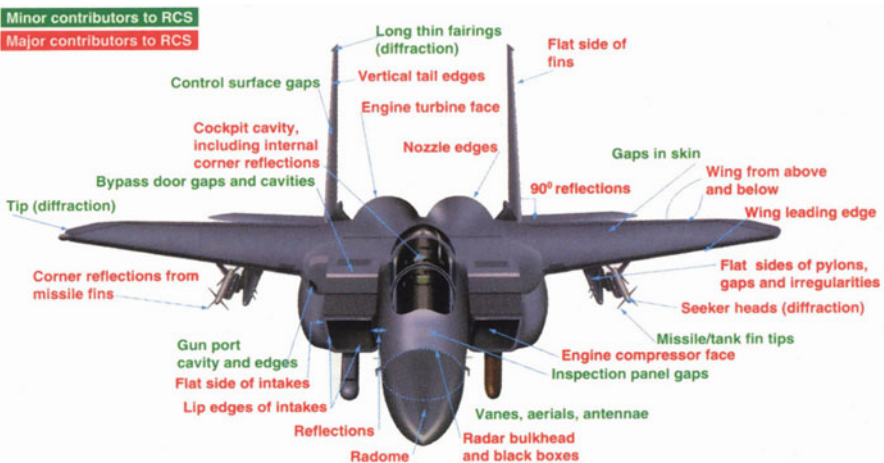
Fig. 4.44 The minor and major contributors to RCS of a fighter aircraft [28]
