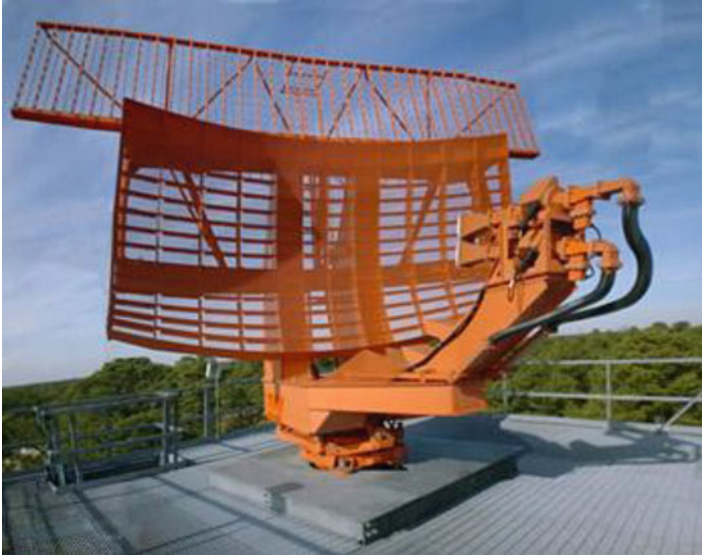
Fig. 2.13 The antenna system of a typical air traffic control radar beacon, the ASR-9 ( www.wikipedia.com )
