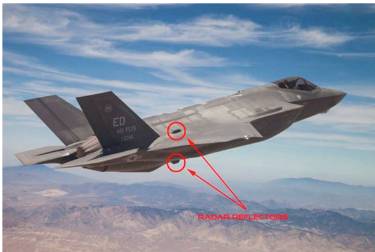
Fig. 3.9 Stealth jet fighter F-35 with the two radar reflectors installed
