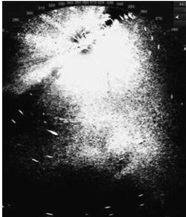
Fig. 1.76 Precipitation clutter with no fast time constant (FTC)
