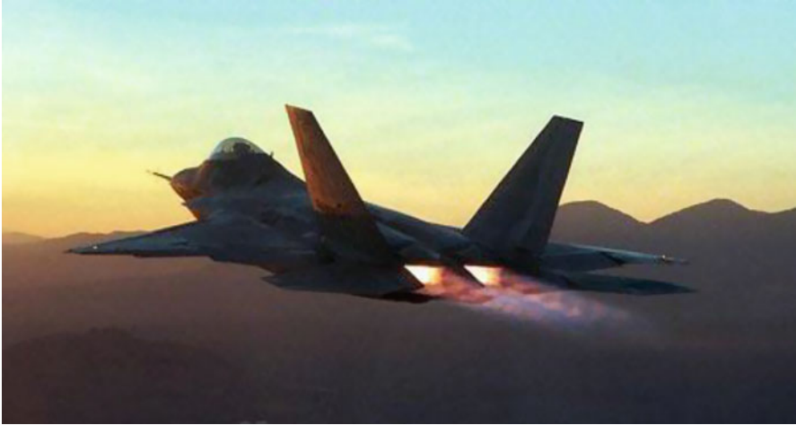
Fig. 4.55 F-22 Raptor’s sawtooth-, wide-, and flat-shaped nozzles to reduce both radar and IR signatures [35]
