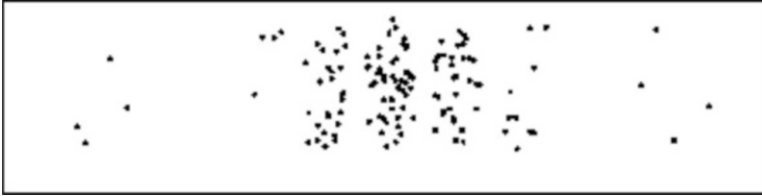
Fig. 1.70 Pattern formed by 2000 electrons on passing through the equivalent of a double slit
